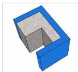
Half shoulder Block to be cut on building site
